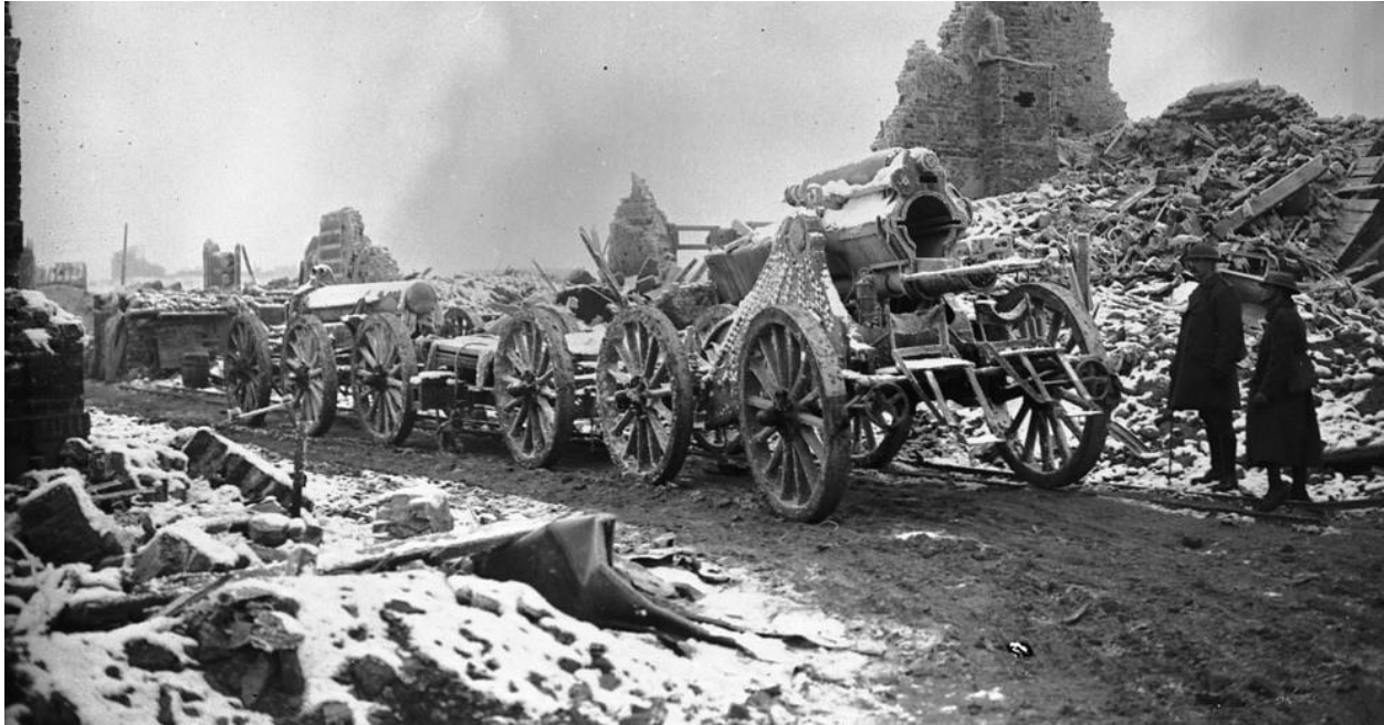
9.2-inch Howitzer mounted in pieces on wagons near Lens, France, Feb 1918. (Library and Archives Canada Photo, MIKAN No. 3395348)
