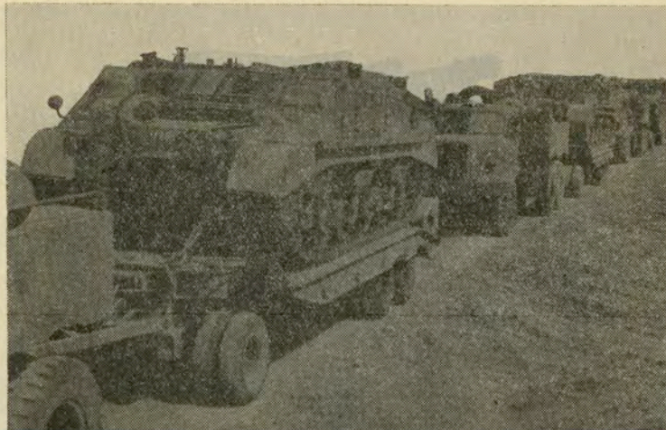
Recovery tanks on 40-ton trailers showing grousers and jib boom stowed on hull nearside
