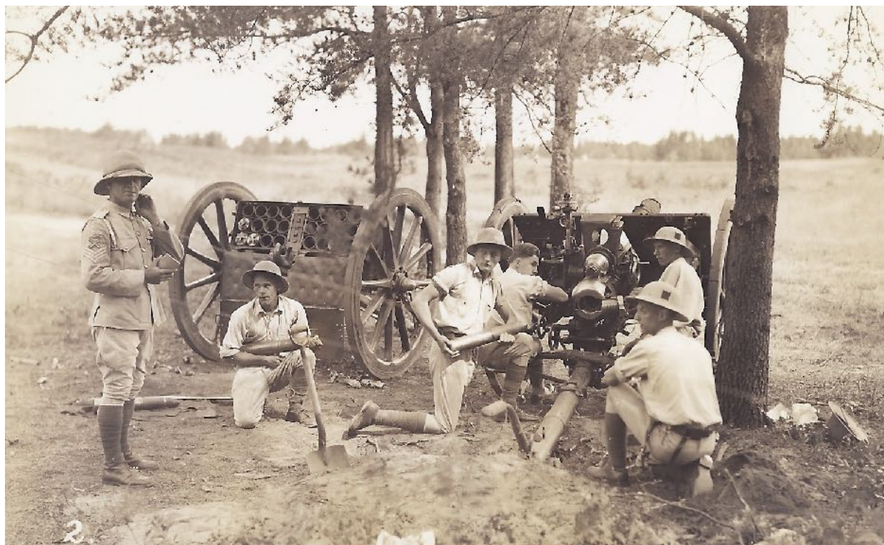
A posed photo of an 18-pounder detachment in the 1930s. From the left: No.1 (sergeant), No. 5 (ammunition supply), No 4 (loader), No 3 (gun layer - the sight can be seen to the right of his head), and No. 2 (close to the gun shield). The man kneeling at the right rear of the trail is probably another ammunition number). The other ammunition numbers would not have been needed during peacetime training. Private collection
