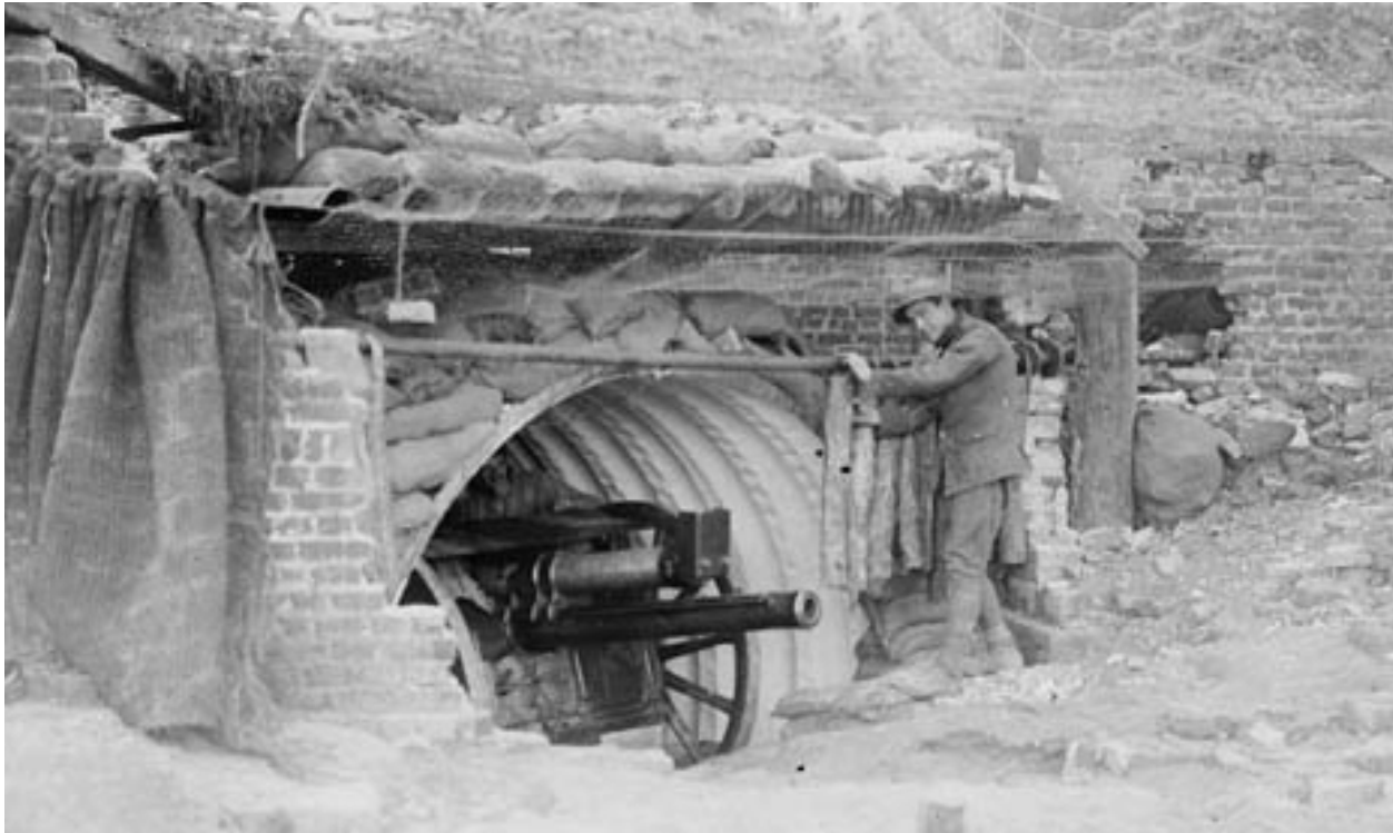
An 18-pounder gun position in France in September 1917. Note the armoured oil reservoir at the front of the recoil cylinder. This allowed for the expansion of the oil in the recoil buffer during intense firing. LAC PA-001876
