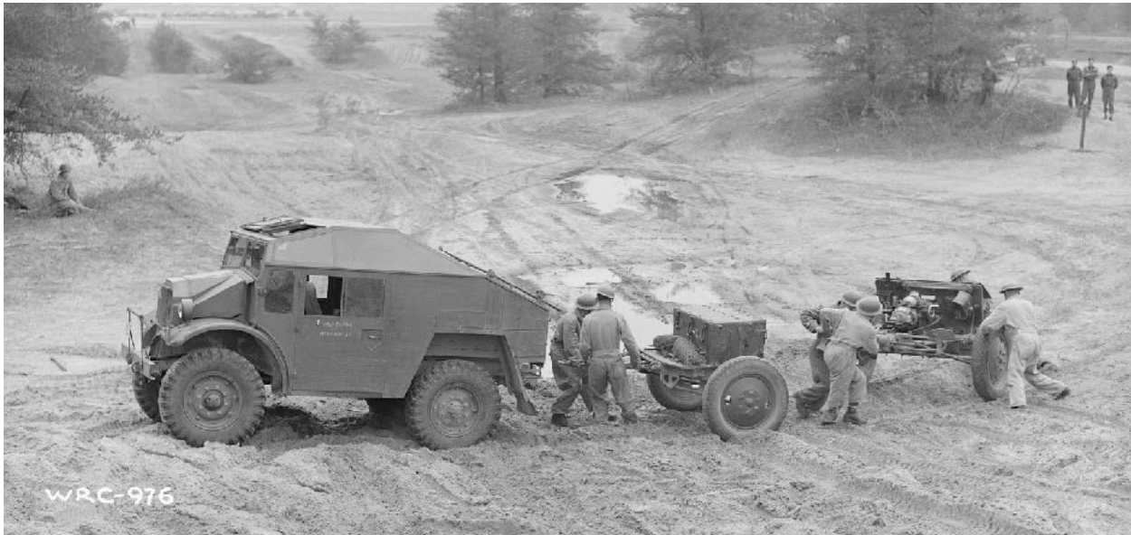
An 18-pounder being used in training in Canada during the Second World War. The gun tractor is a Canadian Military Pattern Field Artillery Tractor, which became the standard towing vehicle for all field guns, starting about 1941. Both the limber and gun have commercial pattern pneumatic tires based on the mechanization standard. LAC 2282983
