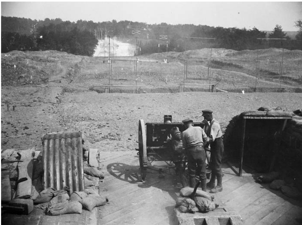
Measuring the muzzle velocity of an 18-pounder on a calibration range in France. LAC a008285
