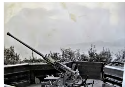
8B - Bofors 40 mm Anti-Aircraft Gun. May 1943. The Swedish designed 40mm Bofors was in Canadian service from 1941-1959. It had a range of 10,800 yards (9900 meters) with a 5,000 feet (1500 meter) effective ceiling. The projectiles weighed 2 lbs (.9 kg). It is shown here in its emplacement forward of the 6" guns. Fort Record Book.
