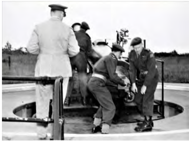
4D – 6 inch Mark VII B.L. Guns on Mk. 2 Mountings. Firing sub-calibre rounds 1947. 15FdMuseum985.101.03
