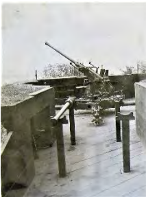
8A - Bofors 40 mm Anti-Aircraft Gun. May 1943. The Swedish designed 40mm Bofors was in Canadian service from 1941-1959. It had a range of 10,800 yards (9900 meters) with a 5,000 feet (1500 meter) effective ceiling. The projectiles weighed 2 lbs (.9 kg). It is shown here in its emplacement forward of the 6" guns with a spare barrel ready. Fort Record Book.
