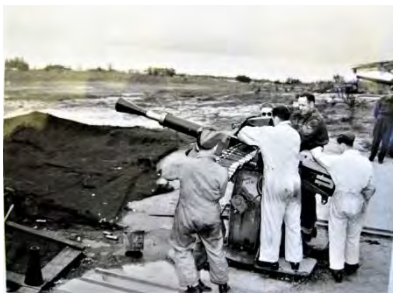
11A – 2 Pdr Naval Ordnance. May 1943. Checking a stoppage in test firing. Fort Record Book
