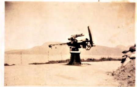
7A - 6 Pounder, 8 hundredweight Hotchkiss Gun. This gun was the standard examination service enforcer in the Coast Artillery Forts. It could fire 25 rounds per minute with a muzzle velocity of 1,818 feet per second (554 m/s) and an effective firing range of 4,000 yards (3,700 m). 15FdMuseum000.15.12
