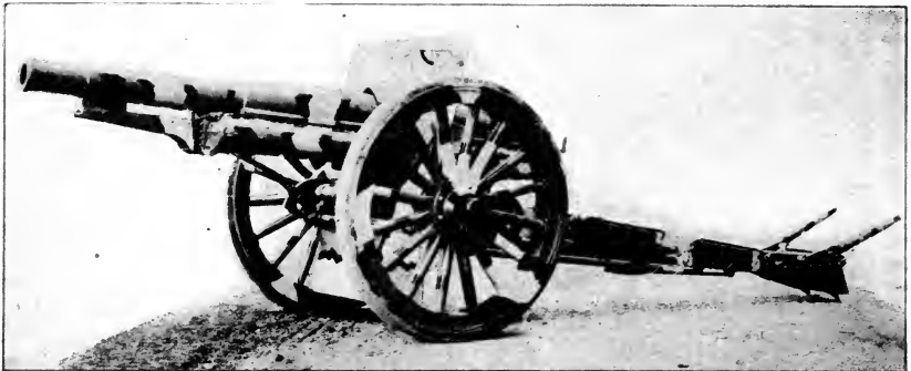
LEFT FRONT VIEW OF CARRIAGE EQUIPPED WITH BAND BRAKES.
