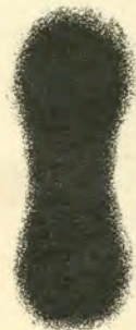
A dumb-bell pattern, heavy at each end and weak in the centre indicates too much pressure.
