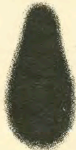
The milk bottle pattern—heavy in the centre means the pressure is too low.
