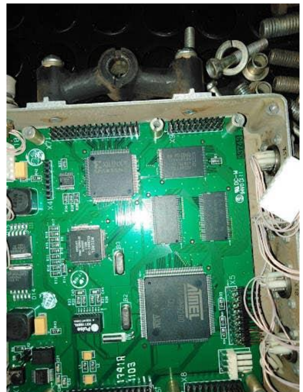
A photo of some of the microchips Ukraine intelligence said it found in the communications system of a Barnaul-T air defense system.
