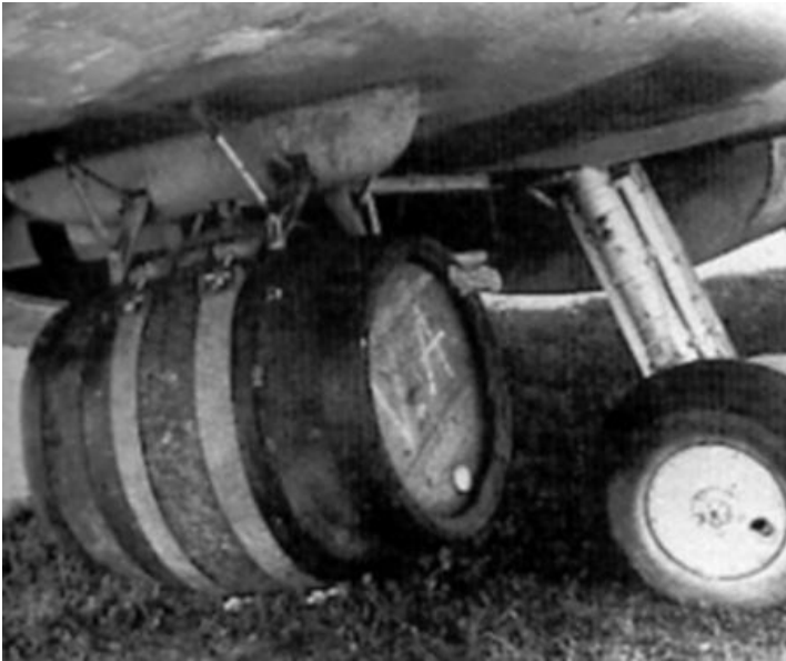
With the larger beer kegs attached to the bomb pylons, the Spitfire had very little ground clearance.
