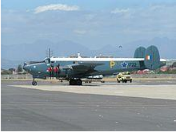
An Avro Shackleton at the South African Air Force Museum - note the contra-rotating propellers, tricycle undercarriage and nose armament
