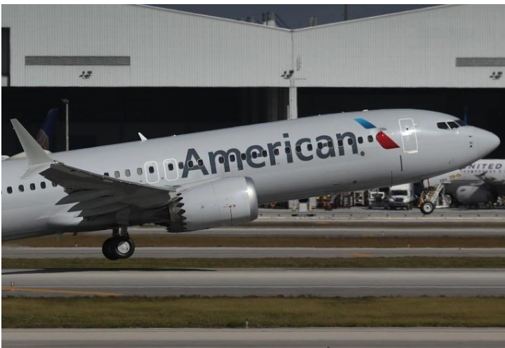
Designers of modern jet engines have taken tips from the owl and designed serrated edges on the back of the engines and wings to make the jets quieter. Research has also shown that adding serrations to the trailing edges of wind turbine blades reduces noise as well. The Boeing 737 Max uses serrated edges along its wings and on the outer part of its engines. Joe Raedle / Getty Images
