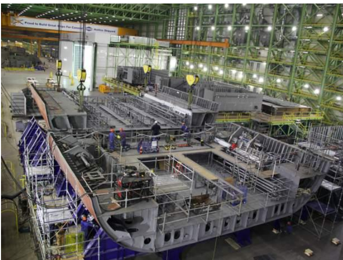
A partially built Arctic Offshore Patrol Ship at Irving Shipbuilding's Halifax Shipyard. Irving Shipbuilding Inc
