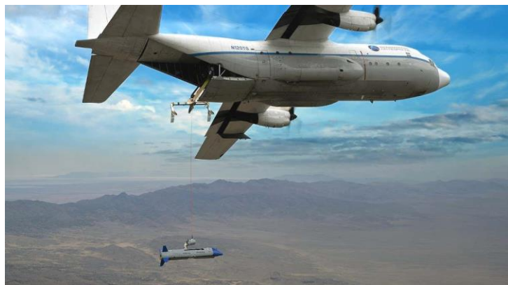
A X-61A Gremlins drone about to be reeled onto a C-130 Hercules during a flight test. LEIDOS
