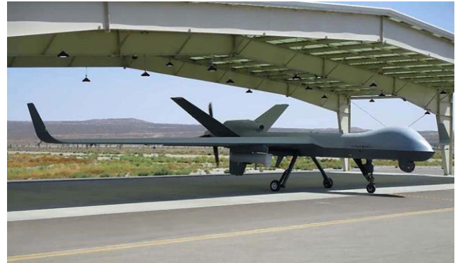
The MQ-9 with the REAP pod. GS-ASI
