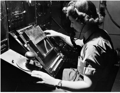
WAAF radar operator Denise Miley plotting aircraft on a cathode ray tube in the Receiver Room at Bawdsey 'Chain Home' station, May 1945.
