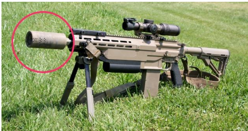
The Next Generation Squad Weapon Science and Technology prototype with "smuzzle" suppressed muzzle brake attached. (US Army/Daniel Cler)
