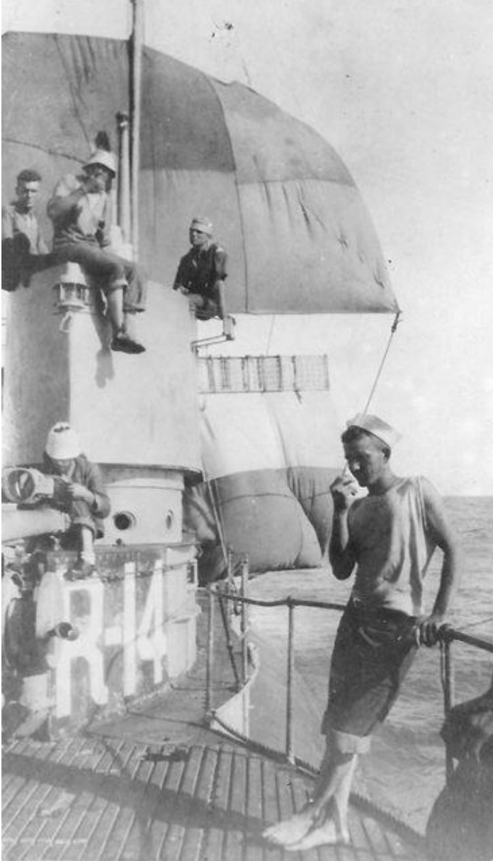
Seen here are the jury-rigged sails used to bring R-14 back to port in 1921; the mainsail rigged from the radio mast is the topsail in the photograph, and the mizzen made of eight blankets also is visible. R-14's acting commanding officer, Lieutenant Alexander Dean Douglas, USN, is at the top left, without a hat. (US Naval Historical Center).
