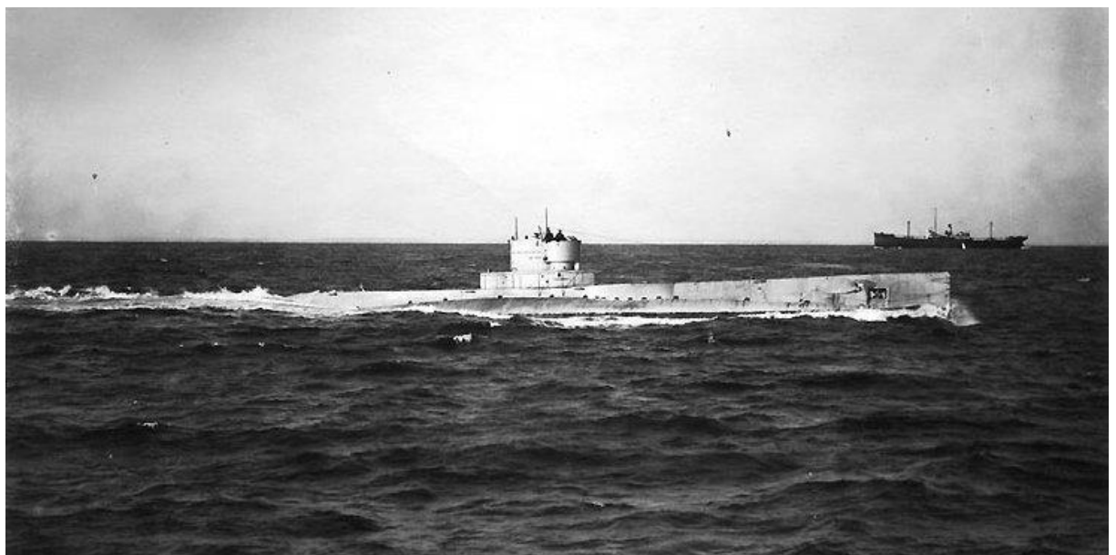
USS R-14 underway, probably during trials in late 1919 or early 1920. Note that her deck gun has not yet been installed. (U.S. Naval Historical Center Photograph NH 102849)
