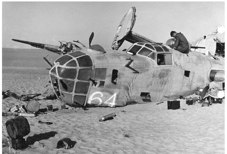
Nose view of Consolidated B-24D Lady Be Good crash site. The plane made a surprisingly good pilotless belly landing and skidded 700 yards before breaking in half and stopping. (US Air Force photo)
