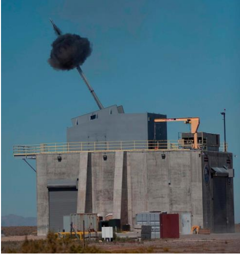
A land-based test of the AGS prior to installation aboard USS Zumwalt. USN
