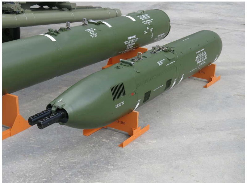
A UPK-23-250 gun pod at the ARMY-2018 arms exhibition at Kubinka outside Moscow. Boevaya Mashina/Wikimedia Commons
