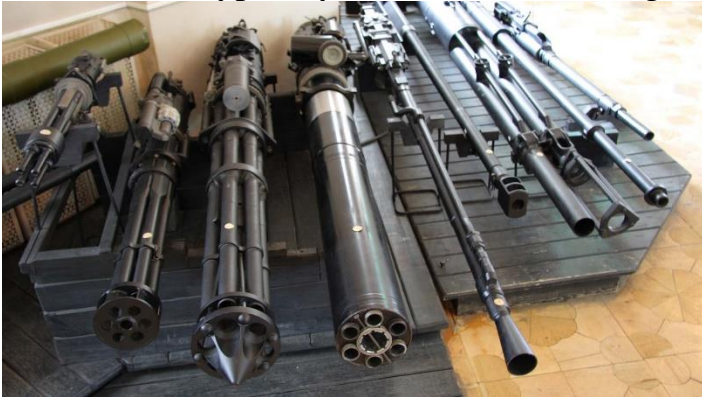
An array of Soviet-designed guns, many of which appeared in podded form. The rotary weapons here are, from left to right: GShG-7,62, GSh-6-23, GSh-6-30, and the naval AK-630.
