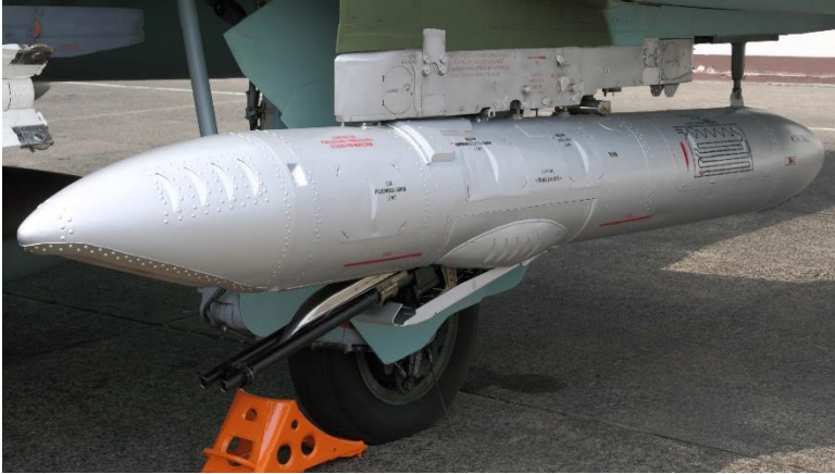
An SPPU-22-01 carried by a Polish Air Force Su-22 Fitter ground-attack aircraft, showing the twin gun barrels angled downward.
