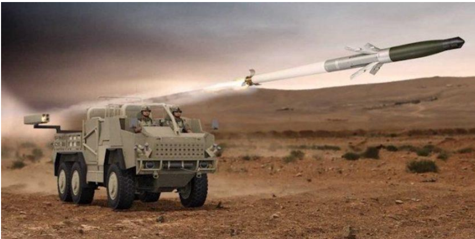
Arnold Defense, a St. Louis-based weapons maker, is working with other defense firms to produce the Fletcher, a weapons system firing 2.75-inch guided rockets that can be mounted on land vehicles and potentially on platforms designed for open-water and close-to-shore operations. Photo via Arnold Defense
