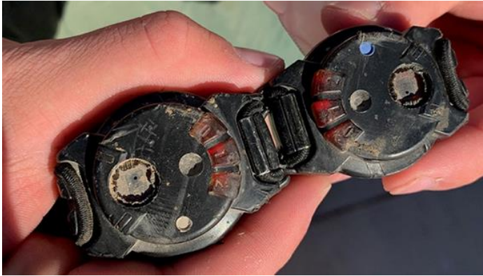
Small, wearable blast measurement gauges show the damages incurred during a recent study of blast pressure exposure at Fort Campbell, Kentucky on Oct. 28, 2022. (US Army photo)
