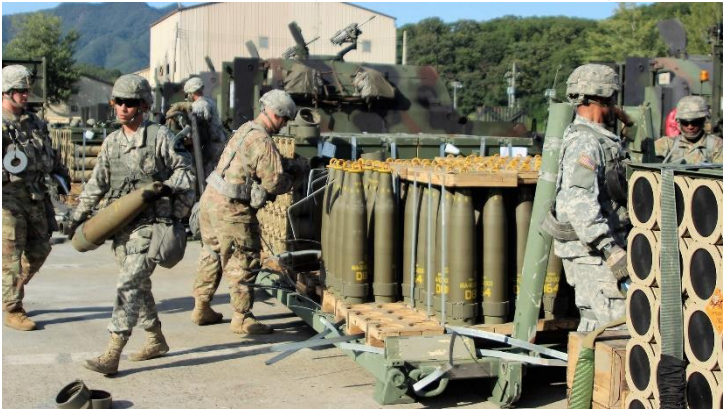
Soldier draw 155mm Base Burn Dual Purpose Improved Conventional Munition rounds, each weighing nearly 100 pounds, and carry into their vehicles during a load exercise. (2 nd Lt Gabriel Jenko/US Army)
