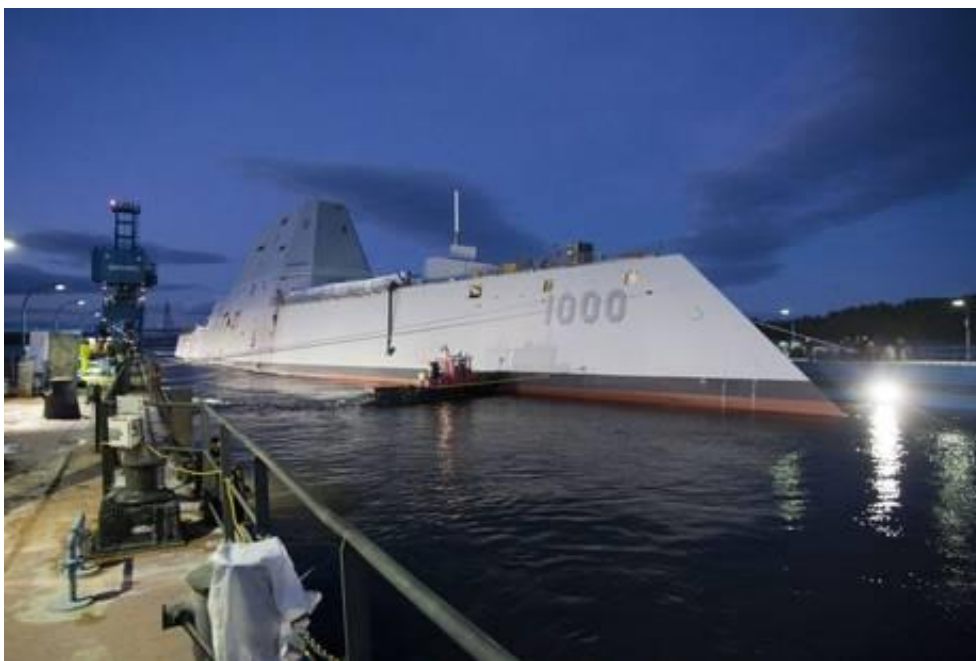
The Zumwalt-class guided-missile destroyer DDG 1000 is floated out of dry dock at the General Dynamics Bath Iron Works shipyard
