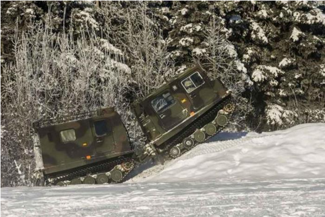
The Small Unit Support Vehicle, or SUSV, that the Army is trying to replace with the Cold Weather All-Terrain Vehicle, or CATV, program. (US Army)
