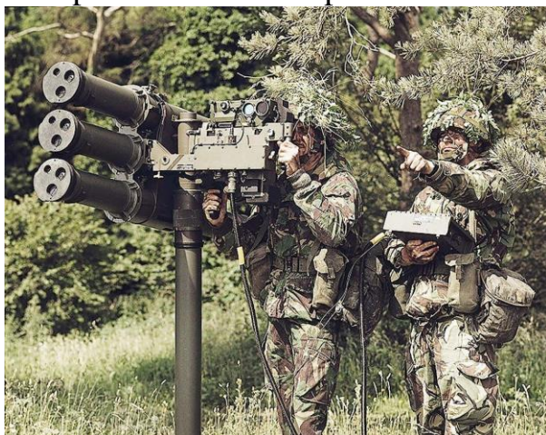
The Starstreak HVM in its Light Role Missile (LML) version with the British Army.
