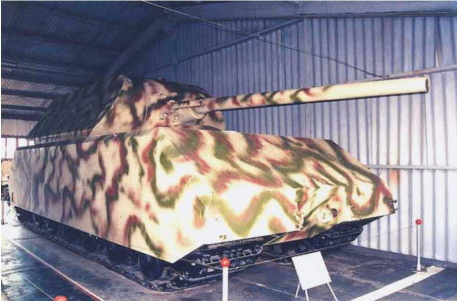
On display at the Kubinka Museum near Moscow, this example of the Maus shows the V2 turret mounted on the V1 hull.
