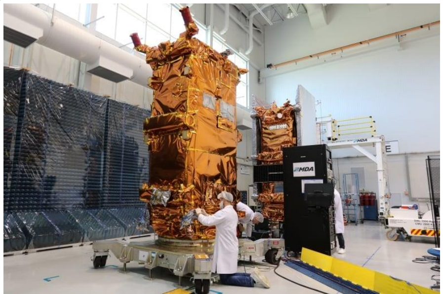
Two RADARSAT spacecraft are prepared for vibration testing in the MDA facilities in Sainte-Anne-de-Bellevue, Que. (Canadian Space Agency)
