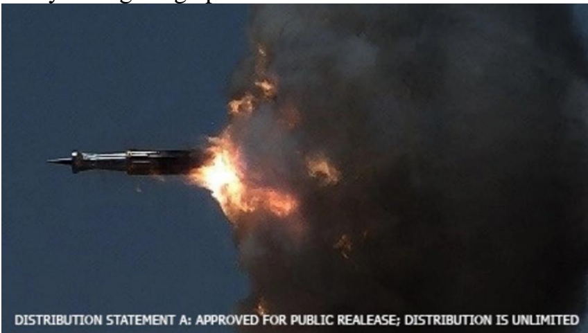
A BAE Systems Sub-Caliber Artillery Long-Range Projectile with Enhanced Lethality concept for the US Army's XM1155 sub-caliber program fired from an Extended Range Cannon Artillery (ERCA) during a recent test at White Sands Missile Range in New Mexico. (BAE Systems)
